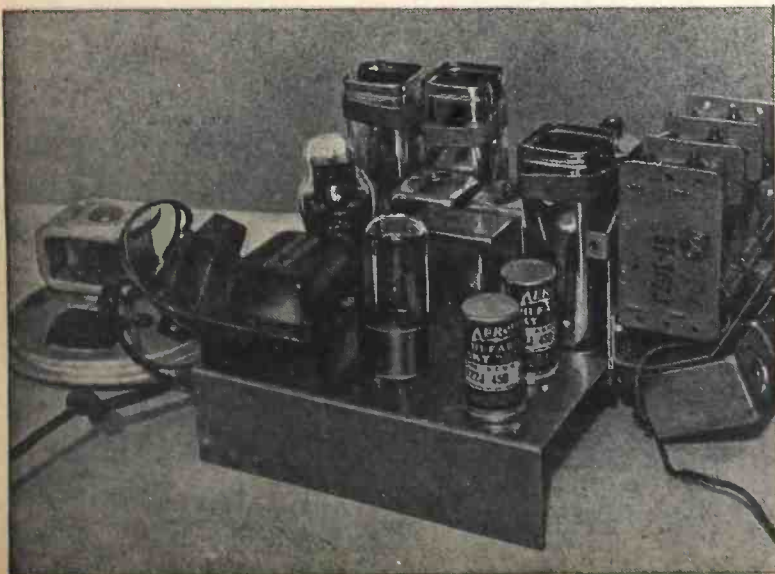
A power supply on a separate chassis made an a.c. radio out of this auto set. Speaker field is filter choke on this particular receiver.
