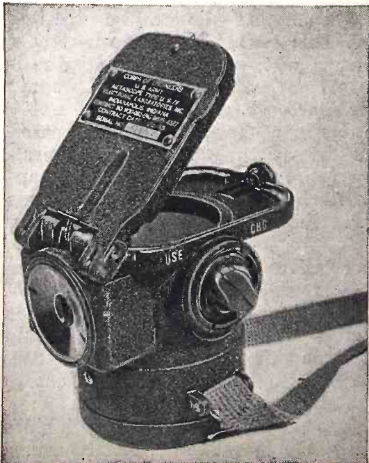
The Metascope, detector of infra-red light.
